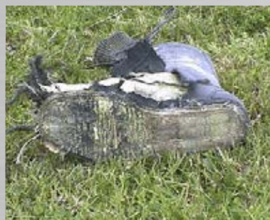
BCB1 Boot after 50g explosion on ball
