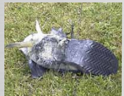
BCB1 Boot after 70g explosion on heel
