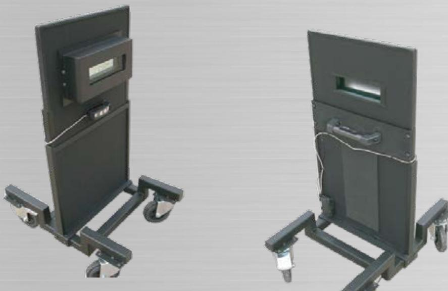
The level IV ballistic shield is a mobile high protection shield which provides multi strike protection from armour piercing rounds, and all lesser ballistic threats. The shield is flat and is constructed from alumina oxide ceramic tiles mounted on a rigid matrix aramid backing. The trolley provides a stable and highly manouverable platform capable of smooth cornering, and rough terrain movement. The included PRO LIGHT Shield Lighting System allows you to operate even in dark environment.
